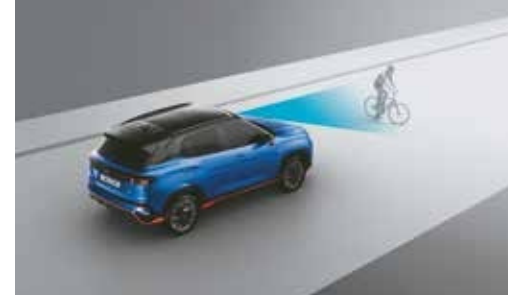
Forward Collision - Avoidance Assist - Cycle (FCA-Cyl)
