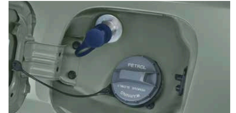
Convenient CNG filling with fast refueling nozzle (near petrol filling area)
