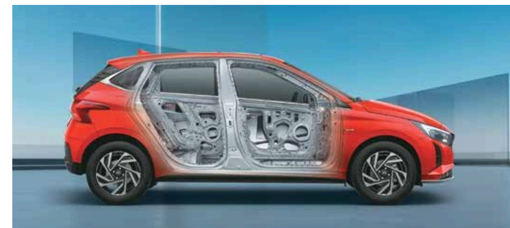
Strong body structure (with AHSS and HSS)
