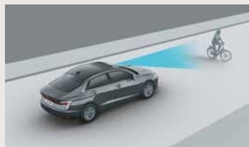
Forward Collision - Avoidance Assist - Cycle (FCA-Cyl)
