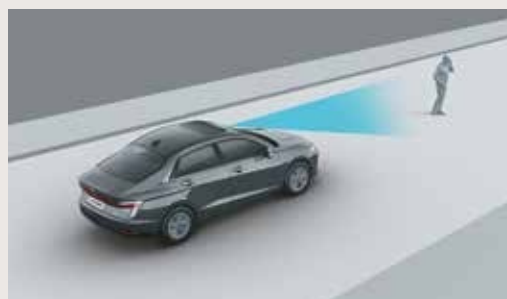
Forward Collision - Avoidance Assist - Pedestrian (FCA-Ped)
